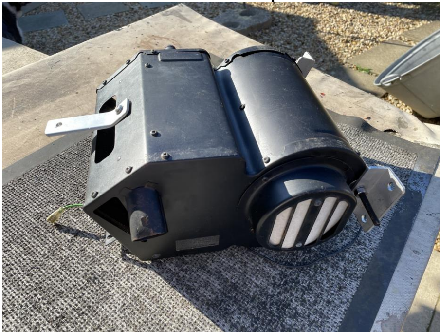
Aluminium brackets in position and control panel removed.
